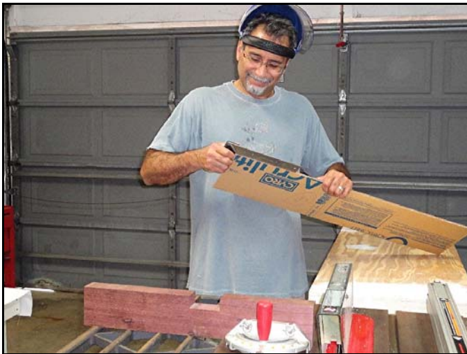
Always check your cuts to be sure that they are square. Waxing the blade also prevents the Plexiglas from melting which can ruin a cut.
