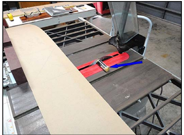
I buy long lengths of Plexiglas with a width a few inches wider than I need so that I have extra material to work with just in case! The secret to cutting Plexiglas is to wax the blade every few cuts.
