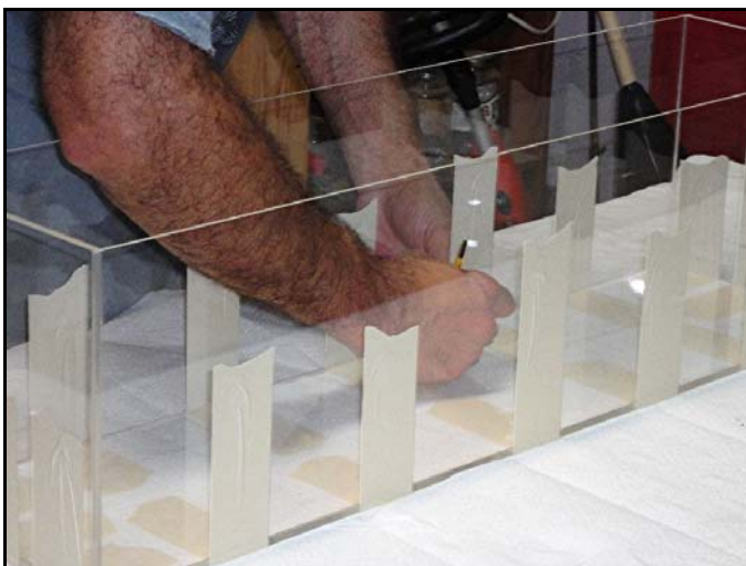
Here again I carefully apply the Tenax-7R glue along the seam line and let capillary action suck the glue along the contact surfaces.
