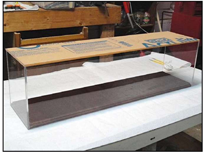
The top gets on final fit check before edge polishing and gluing.
