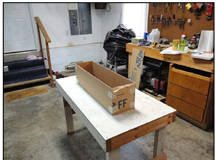
I build the case around the display base. The lengths are cut slightly longer so that the edges of the widths sit against them. I cut the 1st length, then a width then the 2nd length and then the last width.
