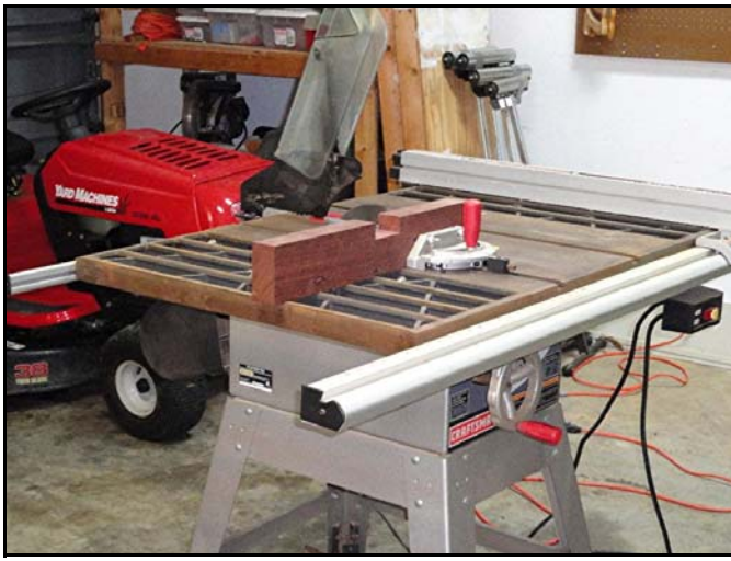
To make display cases you need to be working with a good quality table saw. Mine is a Sears Craftsman 10 inch belt drive saw.
