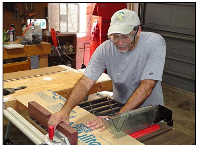
I have found that pulling Plexiglas through the blade works better than pushing it. Always use the blade guard and wear safety glasses or a safety shield. Yep — it was hot in the garage.
