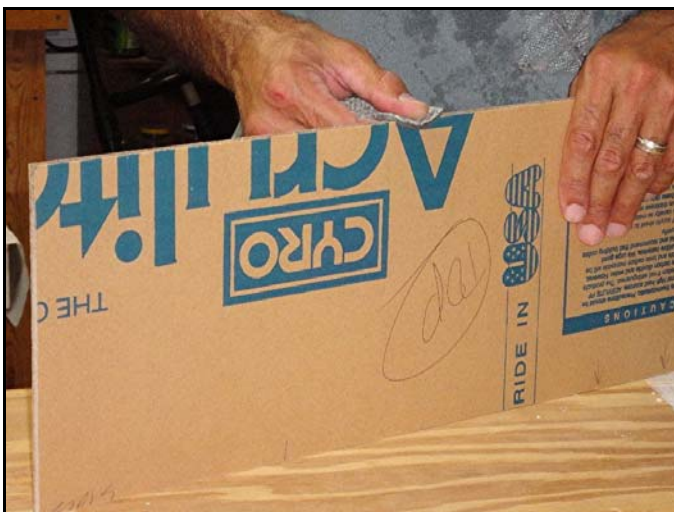
After sanding I polish the edges with 0000 steel wool pads. The steel wool pads polish the edges to an almost transparent surface.
