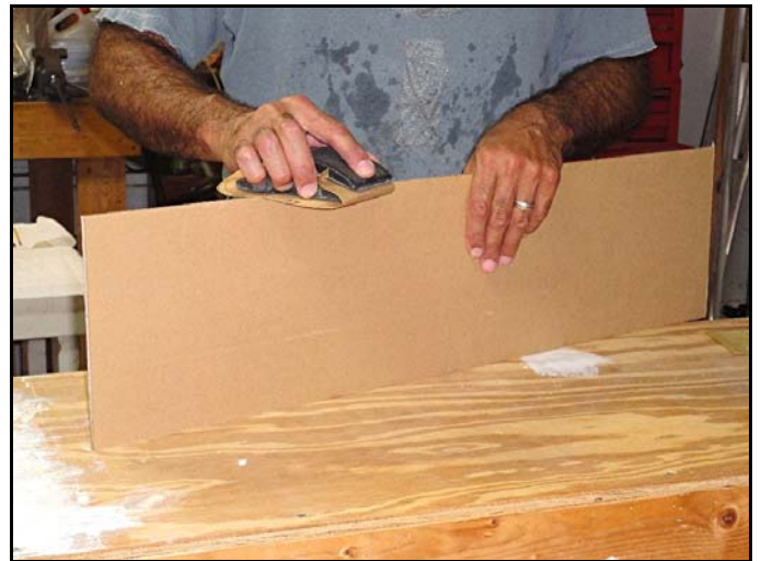
To polish the edges I start with 150 grit sandpaper and then smooth it out with 200 grit. I try to keep the sandpaper block flat against the edge, but I am not always successful.
