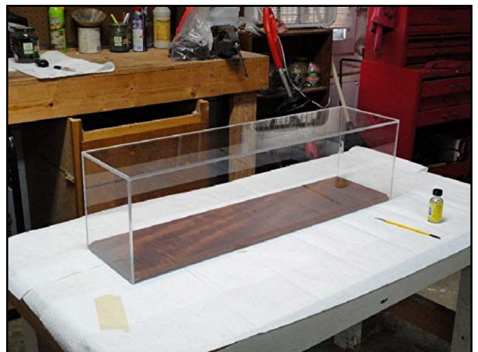
The case is now complete! To remove masking tape glue residue use Windex. To help protect the surfaces of the case against glue splashes cover them with masking tape.
