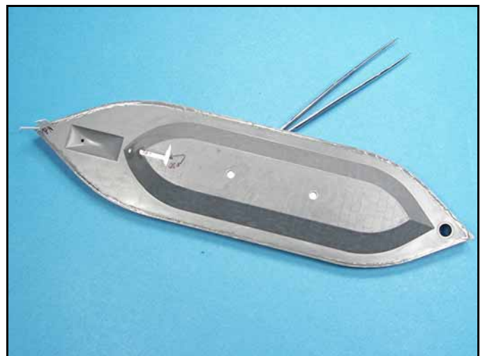
Several layers of plastic were also glued to the inside of the hull to cover the openings for the display base. The increased thickness will provide a better contact surface for the brass pedestals.
