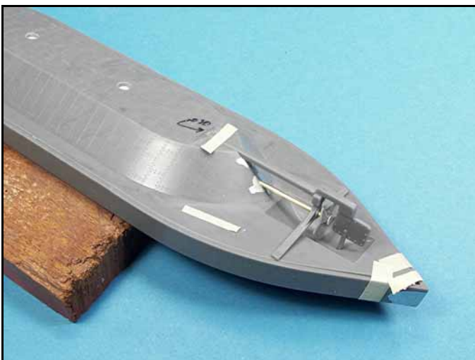
I cleaned up the prop and added a small disk to the end of it to close off the opening. The Skeg and propeller shaft support were glued together to make an assembly. I used brass rod for the propeller shaft.
