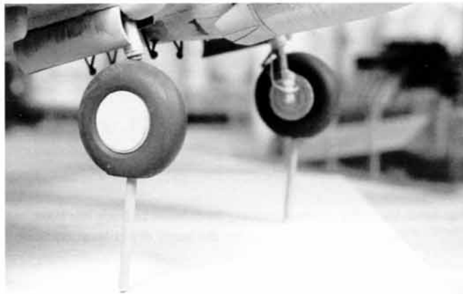
Fig. 6-33. To positively secure a model to a wood display base, drill small holes in the bottoms of the tires and glue pieces of plastic rods into the holes.
