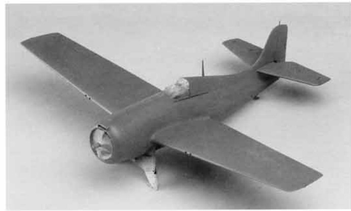
Fig. 6-6. Here the Wildcat has been primed and is ready for the first application of additional masking. Once you have primed the model, check it one last time for flaws and cracks, repair those areas, and reprime. Photo by Glenn Johnson.
