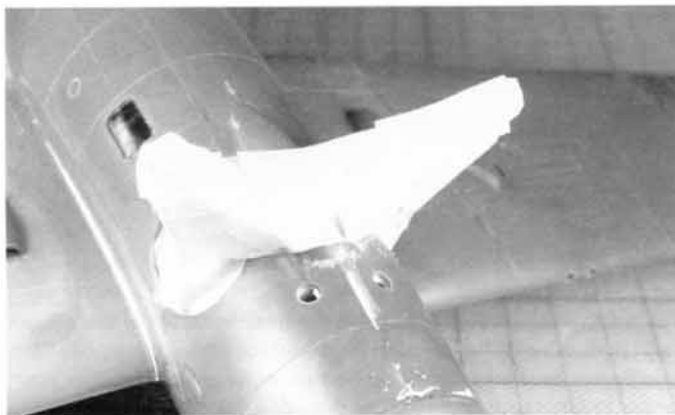
Fig. 6-3. Scotch 3M painter's masking tape cut into small strips works great for masking landing gear.
