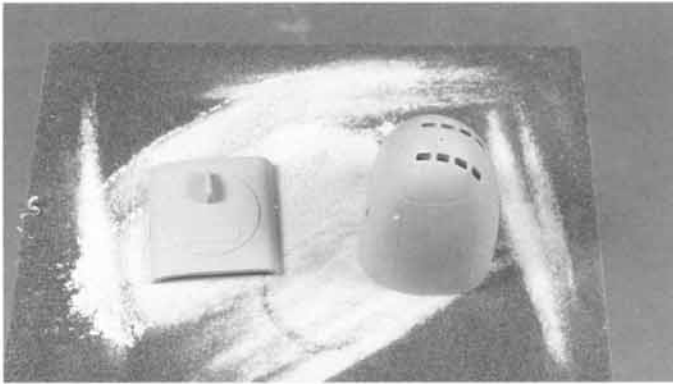
Fig. 2-15. To clean up large resin detail parts and flatten their attachment surfaces, run them across a stationary piece of sandpaper. Use a figure-eight motion or rotate the part to insure that you do not remove too much resin on one side or edge.
