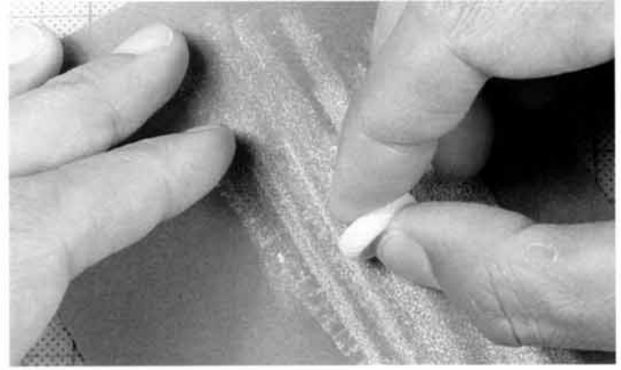
Fig. 2-2. Next, hold the tire flat and run it across a stationary piece of sandpaper to remove the remaining resin.
