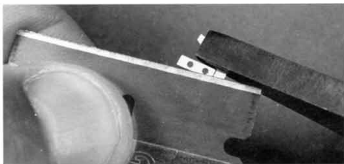
Fig. 2-54. Photoetched cockpit detail sets, especially the Eduard's series, have a lot of small parts that need to be bent into box shapes. The easiest way to ensure good bend lines is to position the part in a set of flat-nose pliers along the bend line and then bend the part using a single-edge razor blade.
