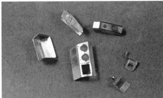
Fig. 2-55. These box shape parts were all bent into shape using a combination of single-edge razor blades, flat-nose pliers, and a set of tweezers. The tweezers were used to make fine adjustments.
