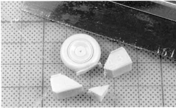
Fig. 2-1. The first step in working with resin tires is to remove the part from the pour blocks. The easy way to do this is to use a razor saw and cut as close to the part as possible.
