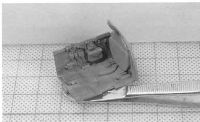
Fig. 2-33. To begin assembling the resin cockpit, work in stages. First set the back and either the right or left side.
