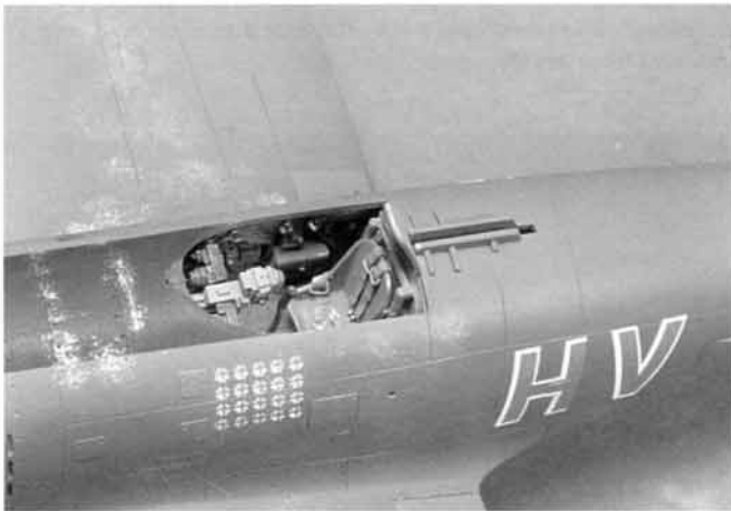
Fig. 2-39. The last step in the assembly of this P47N interior is to add the gunsight, which you do after painting the model, adding decals, and applying weathering. The new cockpit interior greatly enhances the appearance of this model.
