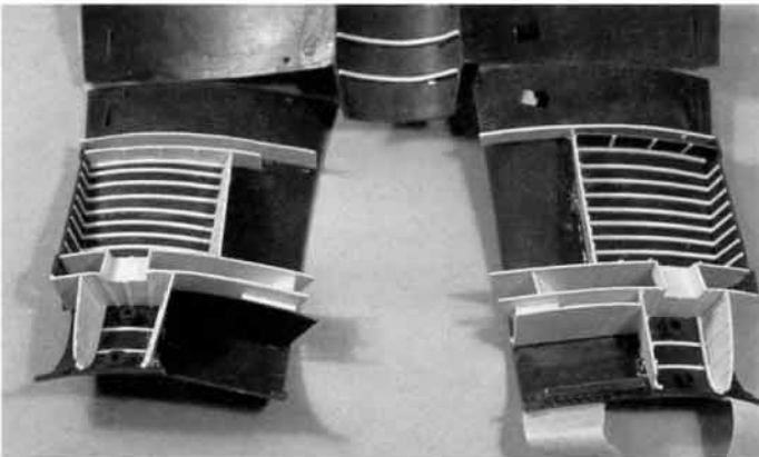
Fig. 1-23. Both sides of the interior landing gear wheel wells of this F4U Corsair are now complete. The secret to duplicating left and right sides is to work with both halves at the same time, completing each step of the construction process before proceeding to the next one. While the parts don't need to be exactly the same, by working in tandem you will get very close.
