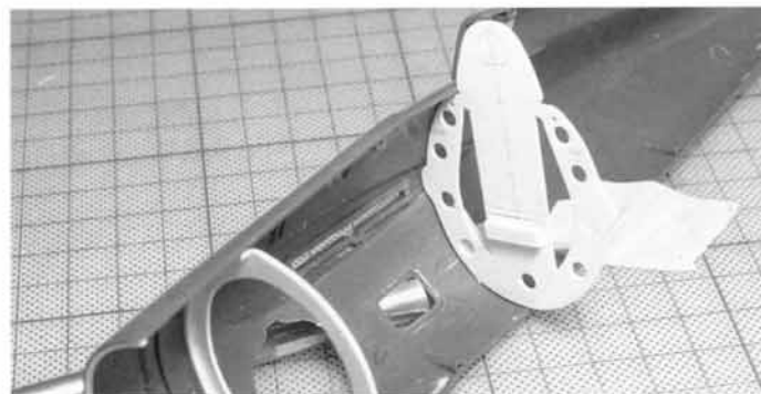
Fig. 1-42. Here the round openings in the bulkhead have been added. To ensure that they are symmetric on both sides, carefully measure and draw the locations of the center points of these openings.
