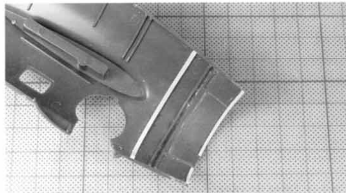
Fig. 1-3. Next use the labeling tape as a guide to glue a small section of Evergreen strip stock into place. This strip stock will act as a lip guide for the contour gauge as well as a positioning tab for the interior part.
