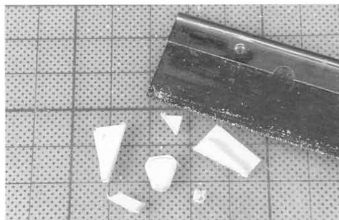
Fig. 1-65. Rough-cut the shape of the throttle quadrant and then sand it to the correct shape.
