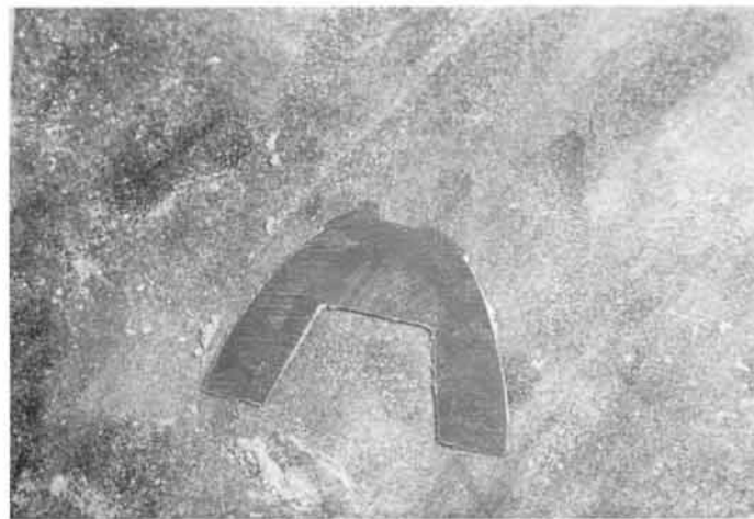
Fig. 1-101. Another way to make a good-looking console is to take the kit's part and sand it down to get it to a thickness at which the Waldron punch tool can punch holes through it. This saves you the time in making a new console, but it works only if the kit's part is an accurate size.
