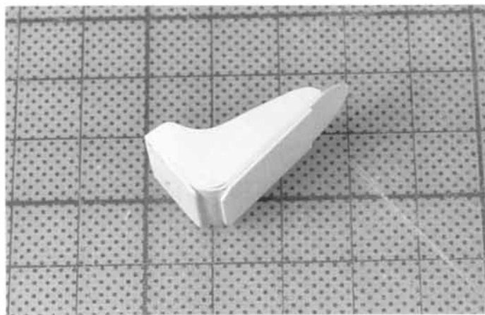
Fig. 1-39. To reinforce the thin plastic sheeting and to represent bulletproof steel plating, glue thicker sections of sheet stock in place on the back and bottom of the seat.
