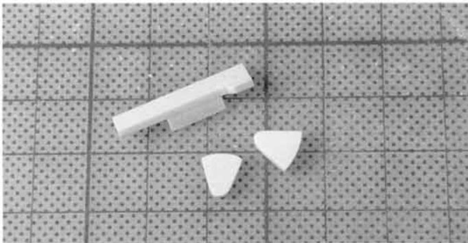
Fig. 1-75. The left side console has been shaped using three different sizes of plastic stock, the larger of which is a small length of Evergreen channel stock. This is also the side where the throttle quadrants will be attached.
