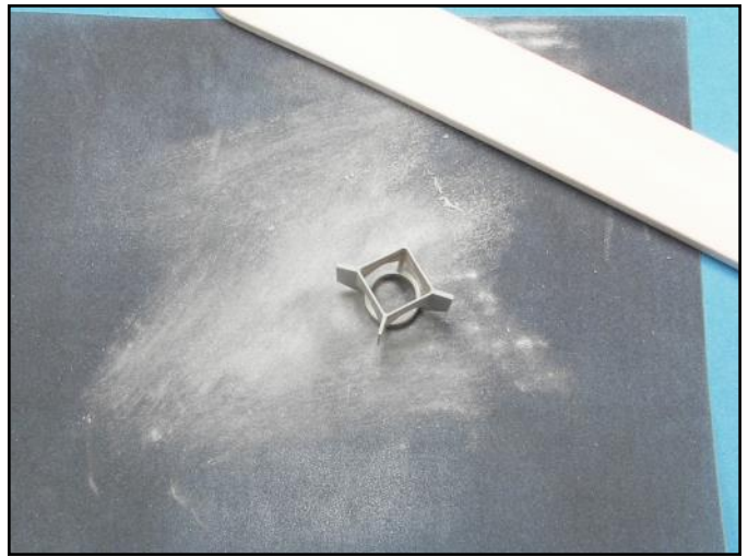
The base of the bomb fin was sanded flat so it would sit correctly on the backside of the bomb.
