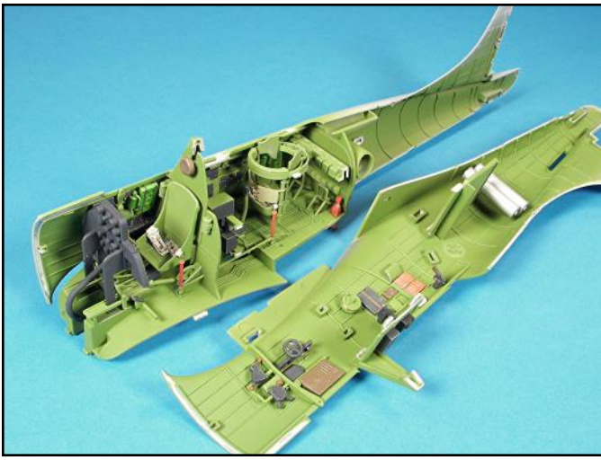
The interior assemblies are complete and it is time to glue the fuselage halves together. Note that the paint that was scraped off the gluing surfaces.
