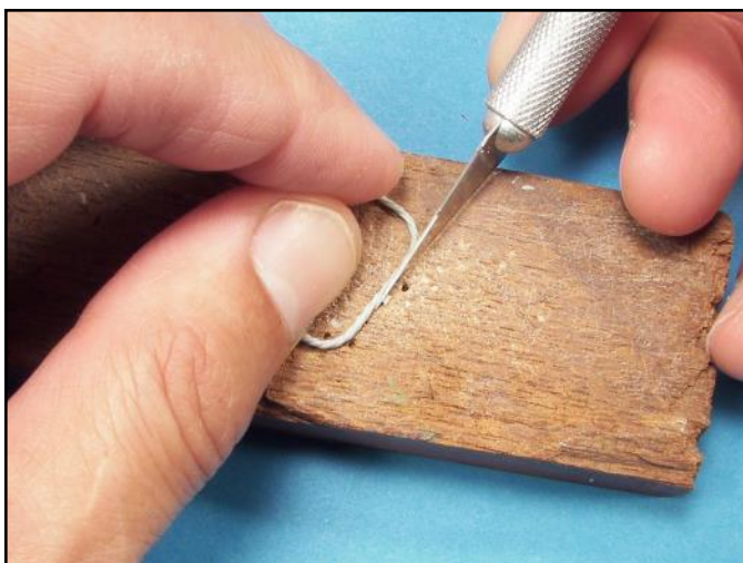
Set small parts onto a small elevated wood cutting board and carefully trim off the remaining tree tabs with the tip of a sharp number 11 X-Acto blade.
