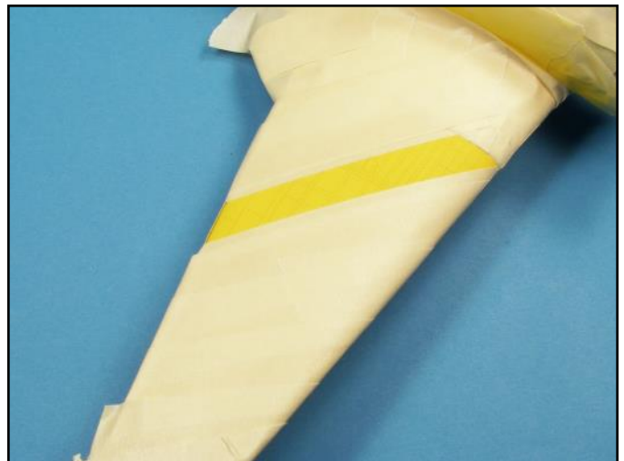
The entire model was then covered with masking tape to ensure no flat red paint dusted onto the surface.
