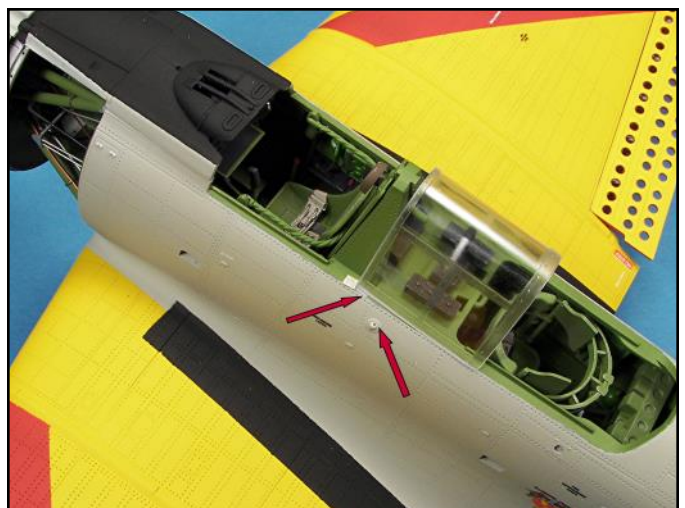
The rear canopy was slightly warped inward and had to be corrected.
