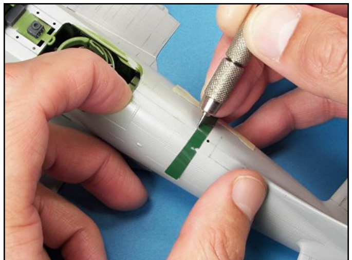
Cutting labeling tape in half makes it more flexible so that it can be wrapped around curved surfaces. The labeling tape edge is perfect for using a scribing needle.
