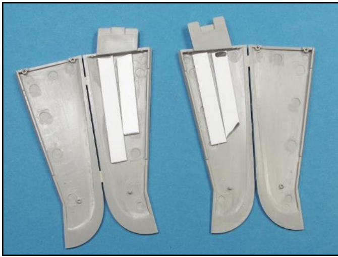
The elevator assemblies were strengthened by laminating sections of .020 inch strips to the interior areas with super glue.
