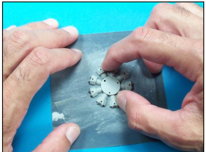
The engine cylinder halves were sanded flat so that the seam line would be minimal.
