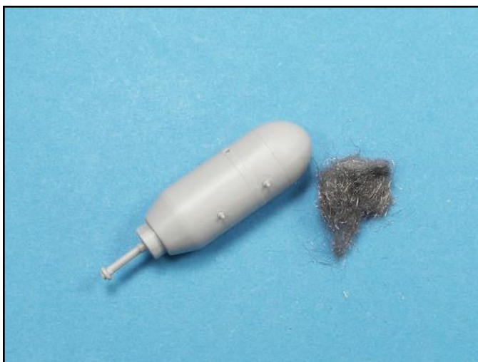
Here again use steel 0000 steel wool to polish the plastic and remove any sandpaper scratches.
