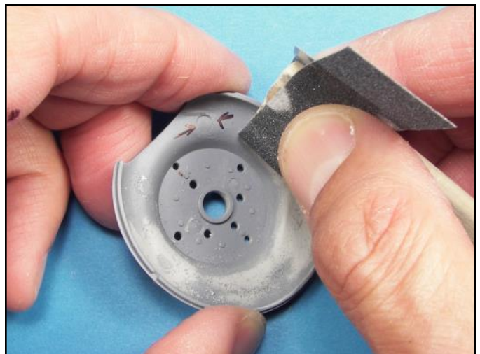
The mold punch out impressions on the inside of the engine heat dissipation shield needed to be sanded out.
