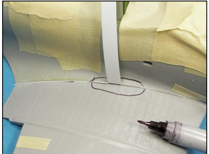
The fuselage to wing attachment areas had some voids that I filled with different thicknesses of plastic strips.
