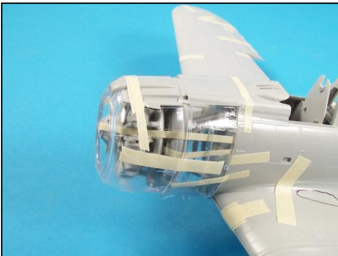
The clear cowling parts around the engine and the engine frame have some fit issues that will need attention if you decide to close up this area.
