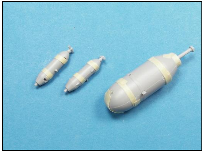
The bombs were taped together and beads of super glue applied around the perimeter of the parts.
