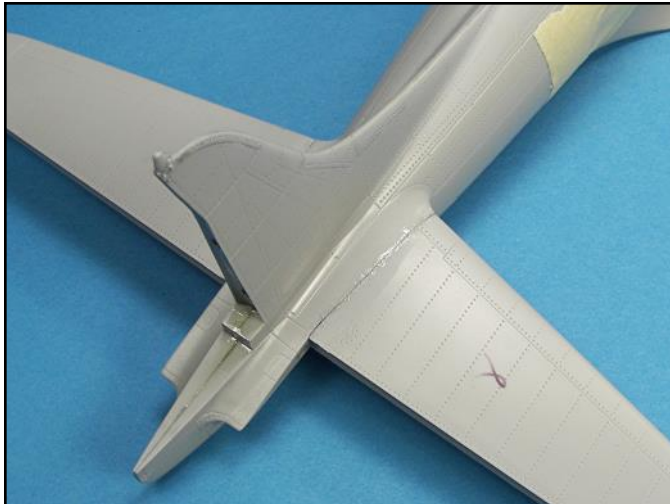
The elevator seam attachment to the fuselage had a very good fit with a minimal seam. The super glue was applied with a thin wire applicator.
