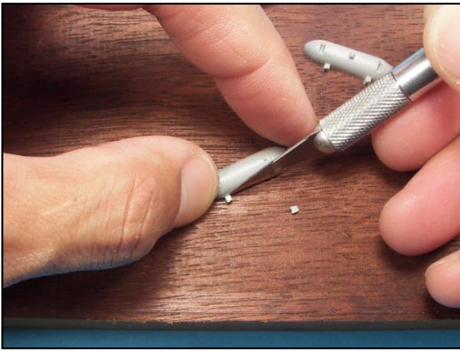
The wood cutting board is also ideal for trimming off excess tabs on parts that have a flat surface.
