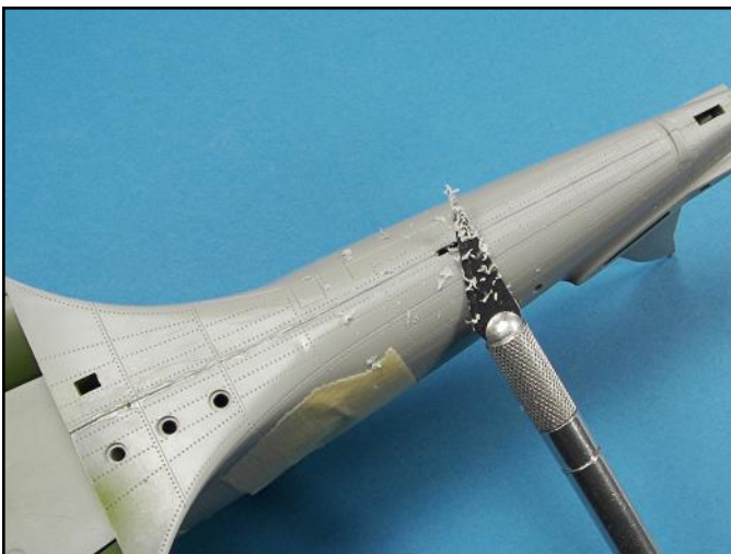
The super glue was carefully scrapped flat and then wet sanded smooth. The fuselage halves fit very tightly together and only required two applications of super glue.
