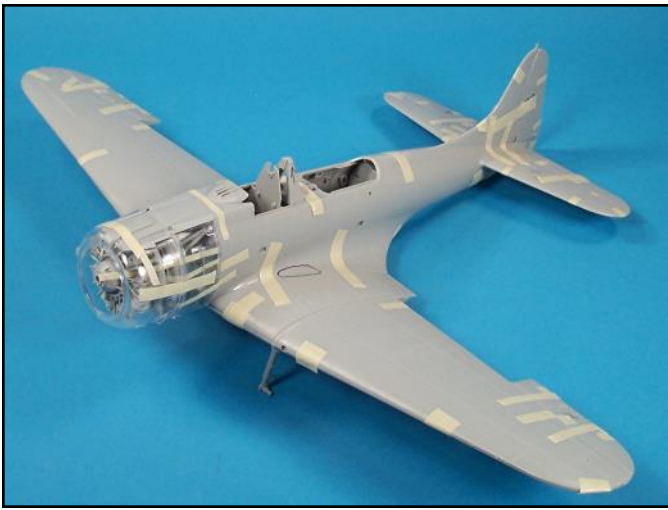
Taping all the major parts together helped identify fit challenges some of which were noted on the instructions and others were marked on the kits surface.
