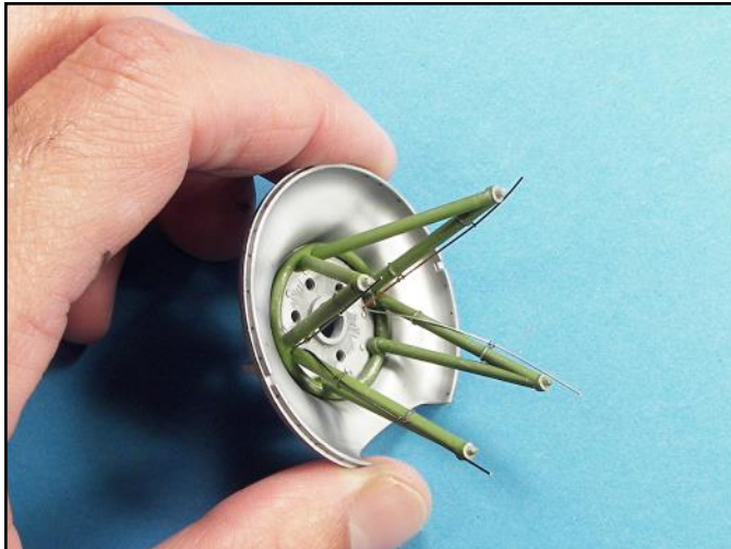
The engine frame is attached to the heat dissipation shield after carefully scraping of the paint from the gluing surfaces. Wiring has also been added.
