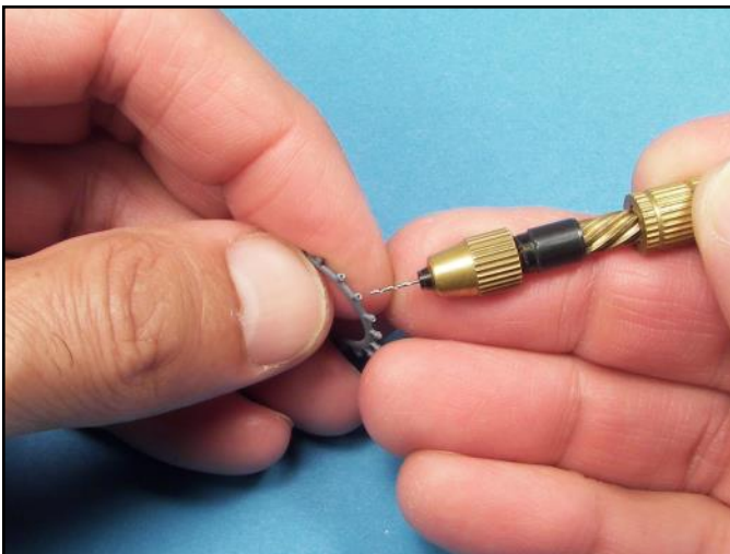
The spark plug wire locations were then carefully drilled out so that brass wire could be inserted into the holes and glued into place.
