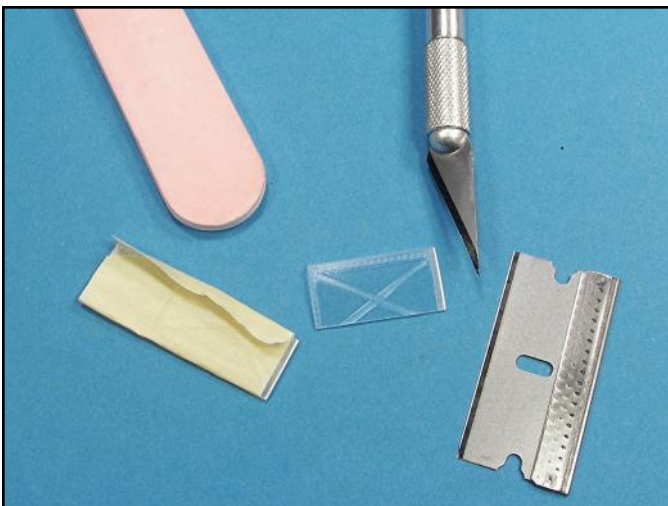
The clear areas were masked to protect them and then the plastic strips were cut to length.
