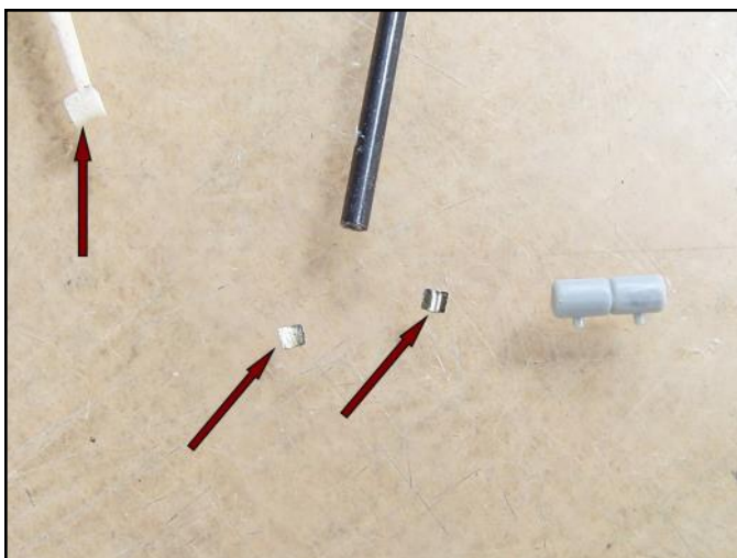
These small name plates were shaped by rolling a Drill bit end across the part. Use a slightly smaller diameter for rolling so that the photoetch parts will fit snugly into place.
