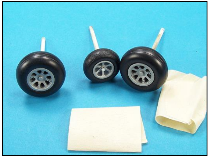
The wheel rims were airbrushed with metalizer aluminum and then glued into place. The flexible tires were perfectly cast, however they were dust magnets. Masking tape was used to remove the dust.
