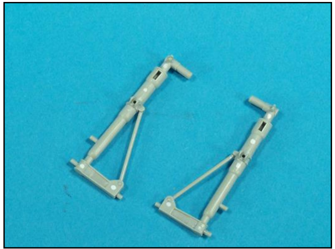
The landing gear had round depressions. I drilled the depressions to a slightly deeper depth and then filled the holes with a corresponding diameter rod. The rods were then cut and sanded smooth.
