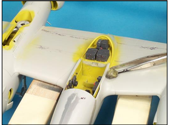
The seam between the cockpit tub and the electronics shelf was carefully filled with tiny drops of super glue and then scrapped smooth. I used a tiny ball of 0000 steel wool to polish the plastic and smooth it out.
