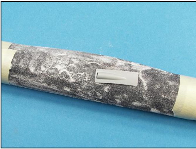
The air scoop panel was thinned out by running it across a wood dowel wrapper with sandpaper.
