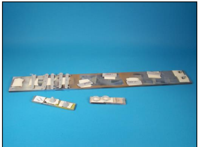
The flaps, landing gear doors and other parts were attached to a length of balsa wood and then primed.
