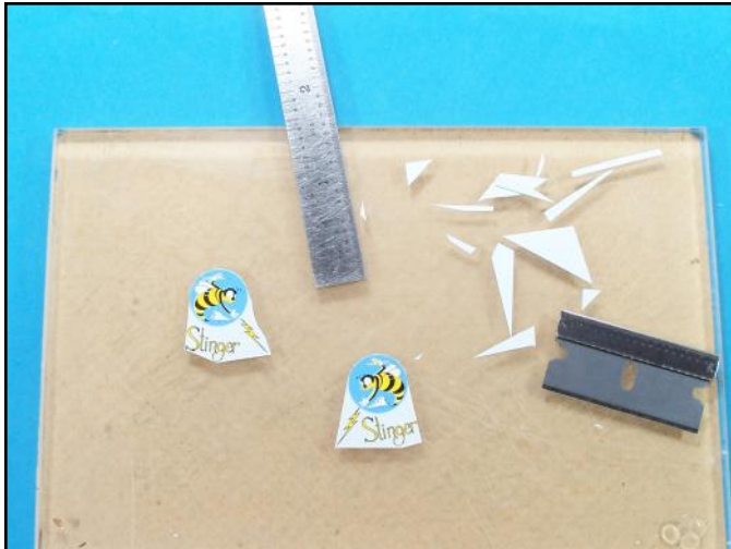
Larger decals can also benefit from removing as much clear film as possible.
