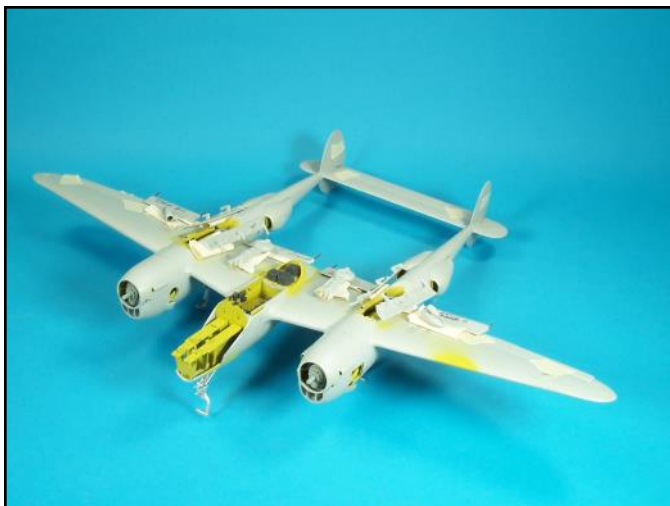
Since I planned to fill the nose with weight I started taping parts at their approximate locations on the upper wind to help determine the proper amount of weight that will be needed.
