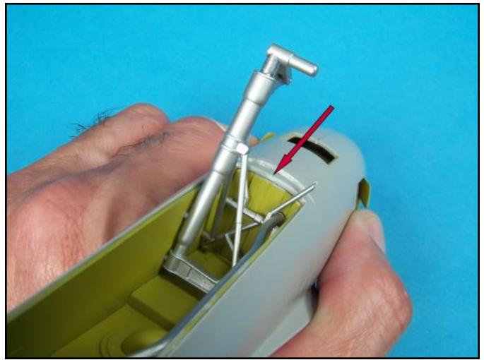
There were tiny voids between the bottom areas of the landing gear bays and the booms. These areas were filled with white glue applied with a .015 diameter stiff wire and contoured with a damp Q-Tip.
