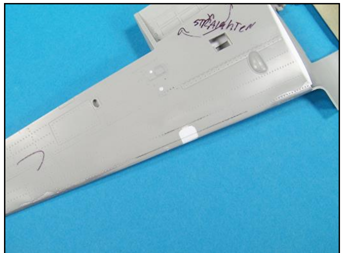
The filled wing lights are now complete and the rivet detail has been restored.
