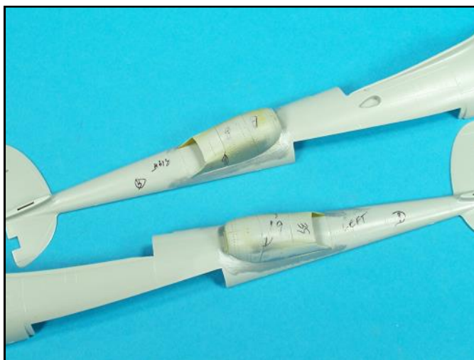
Silver paint was applied to identify any flaws, which were then fixed.
