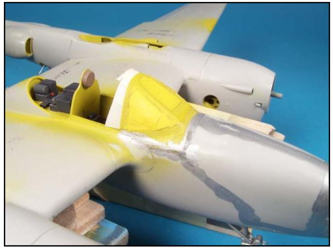
Several iterations of super glue applications and wet sanding were needed to fill the seam between the windscreen and the fuselage.
