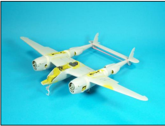
The booms and elevator tail were taped into place, minor adjustments were made and then the port boom was glued into place first.
