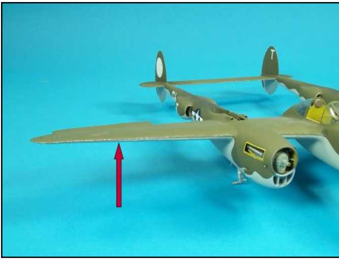
I used a small flat brush to apply tiny amounts of silver paint along the leading edges of the wings and around the engine openings.
