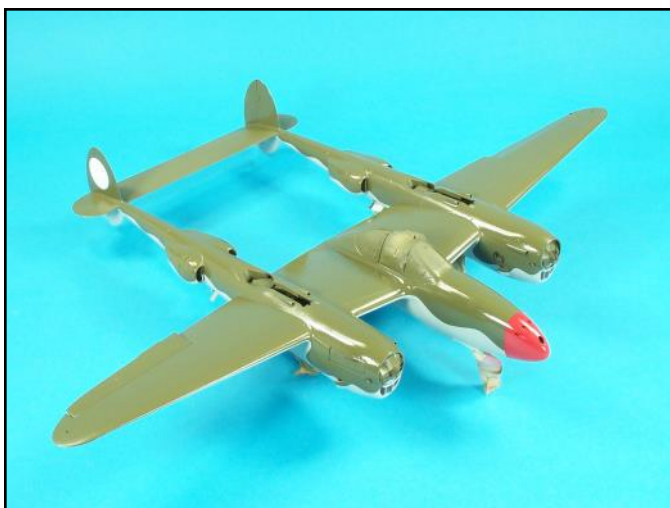
The entire surface of the aircraft was given a coat of clear gloss for the application of the decals.
