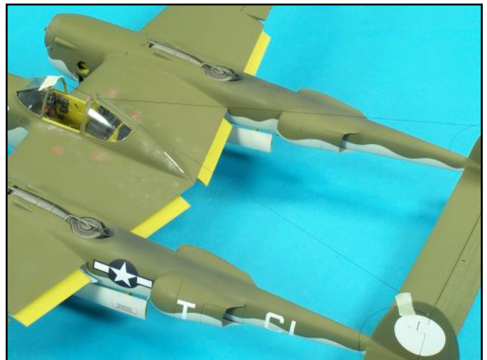
I drilled a hole through the canopy and through the tails using a .0136 (number 80) drill bitt for the antennas.
