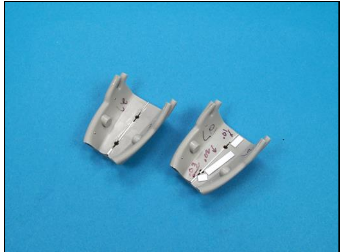
The engine saddles/air ducts needed extra plastic strips to close up the voids. The thicknesses ranged from .010 to .030 inches.
