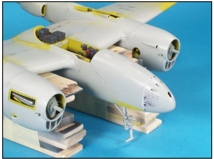
There are misalignments between the upper forward fuselage panels and additional voids along the seam area where the forward fuselage halves meet the lower fuselage.
