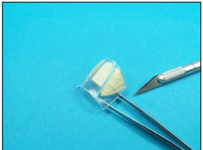
Smaller sections of masking tape were added to fill in the areas outlined by the masking tape.
