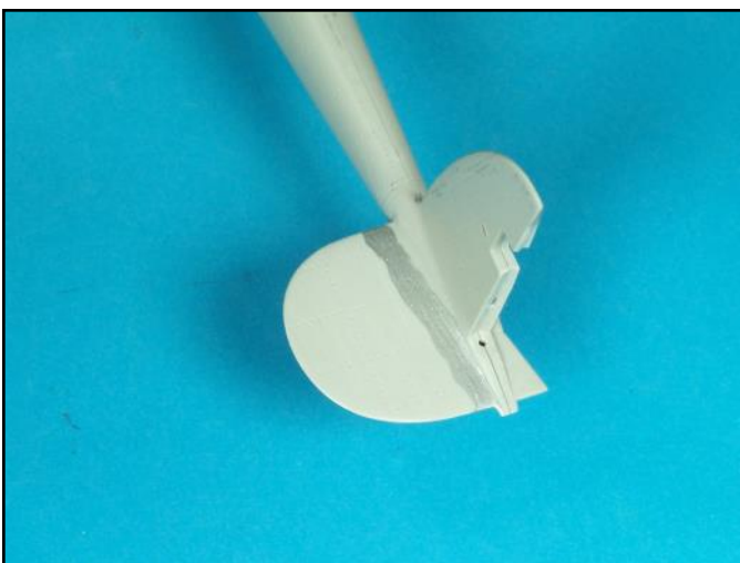
The voids were carefully and lightly sanded smooth and silver paint applied to check for flaws.
