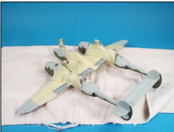
The areas around the interior flap areas were masked off and then zinc chromate was airbrushed at 15 PSI.
