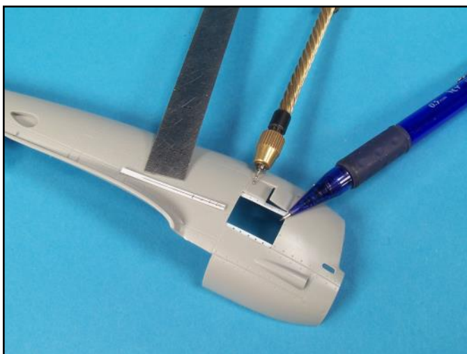
Interior framing for the access panel quick release fasteners was made from .015 inch thick strips. The holes were measured, marked and then drilled out. I also cleaned up and thinned the already opened vent flaps.
