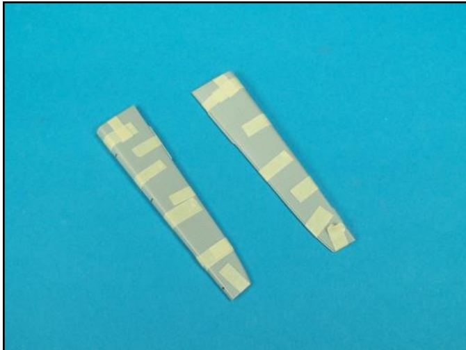
Tiny beads of super glue were applied along the seam lines of the ailerons between the tape. After the glue dried, the tape was removed and additional glue was applied. The seams were then carefully scraped and sanded smooth.
