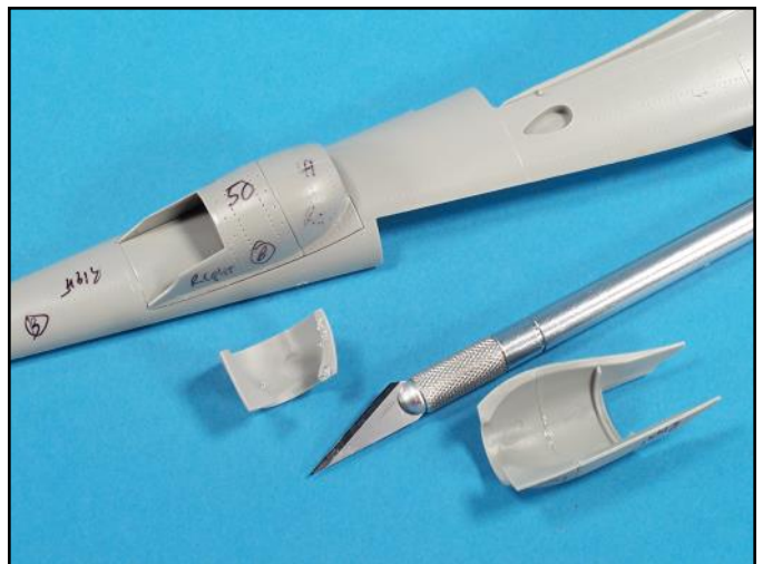
The gluing surfaces of the boom side scoop parts had to be flattened and adjusted to get them to fit into the depressions on the boom surfaces.
