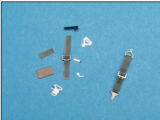
These lap seat belts have several pieces and you have to be very careful when bending the ends of the belts for the locking buckles.
