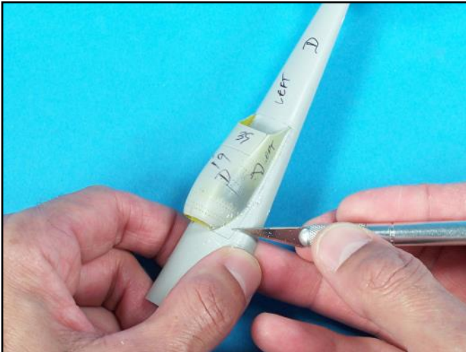
The seams were filled with super glue and then the edges were carefully scraped flat. Be careful not to let the tip of the blade gouge the air scoop.
