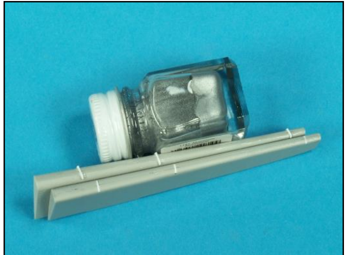
The inside areas of the ailerons had grooves for hinges. These were filled with plastic strips.
