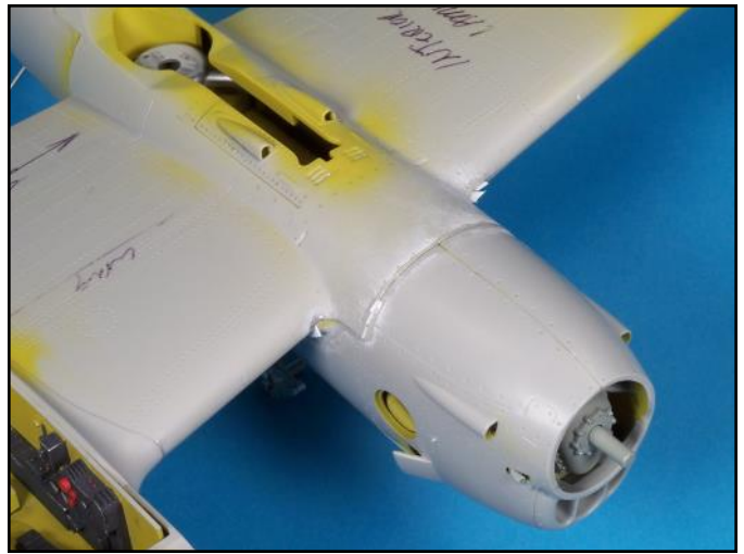
There were tiny voids between the boom and wing connections that were filled with different thicknesses of plastic. It took several applications of super glue to fill the seams. The seam lines were scraped and wet sanded smooth.
