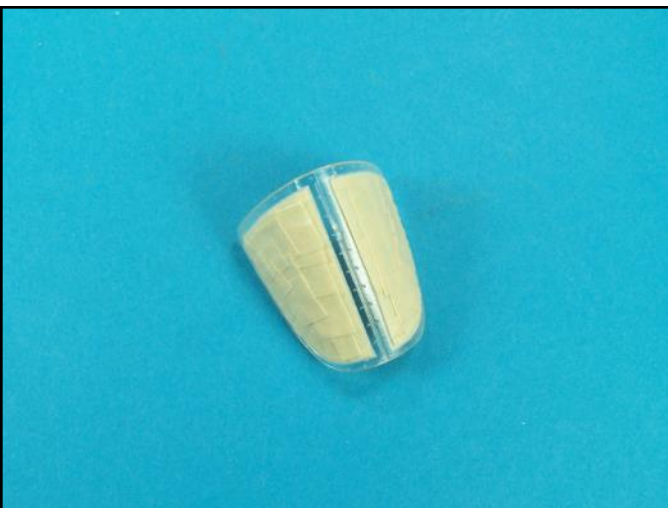
The exterior area of the aft canopy was masked first.
