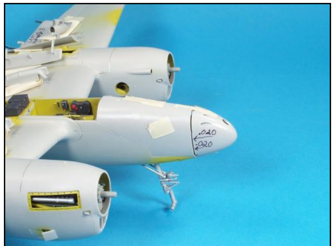
I also taped the nose and the forward fuselage halves in place to check the fit and made notes on the parts. There were voids on these parts that will need to be filled with plastic strips once they are glued into place.
