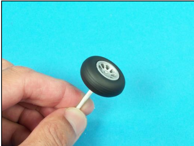
Once the dust was removed with masking tape, they were then immediately airbrushed with a clear flat finish to seal the flexible tires and tone down the metalizer color.
