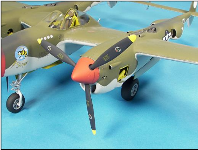
The propellers now have a tight fit. They were attached with tiny drops of Testors tube glue.
