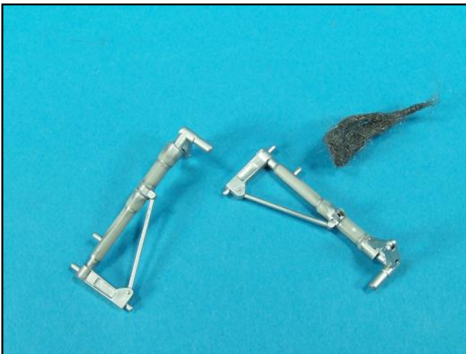
I painted the landing gear with silver paint to check for additional flaws. Having found none, I polished the plastic with 0000 steel wool.
