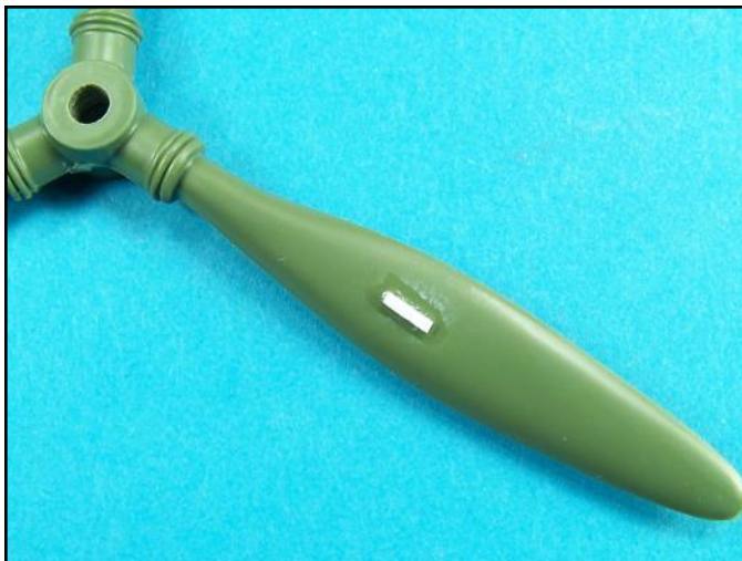
Revell P-38 propellers had a better shape than the kit's propellers, but each blade had a depression, which was filled with a small strip of plastic. The surface was then wet sanded smooth and then primed.
