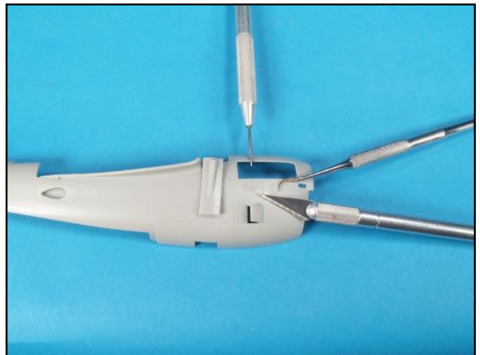
To display some of the engine on each boom, I carefully cut out an access panel on each side of the outside booms. I then thinned the plastic around the cut out areas by scrapping the surface with a number 11 X-Acto blade.
