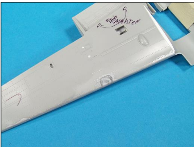
Note the additional super glue applied along the seams after silver paint was applied to detect flaws.
