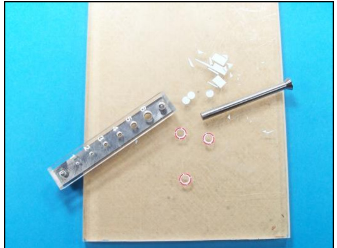
The round circles around fuel ports can sometimes silver so to prevent this from occurring, use a Waldron Punch Tool to remove some of the clear film from the center area.
