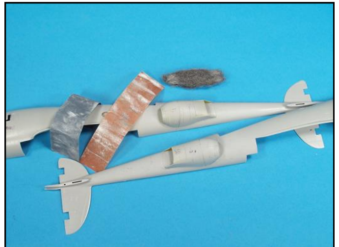
The surfaces on the air scoops and the surrounding surface of each boom was carefully wet sanded smooth and then polished with 0000 steel wool.
