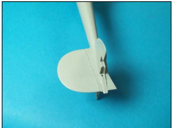
The outer elevator wings were glued into place with Testors tube glue so that minor adjustments could be made to their positioning. The voids were filled with super glue.
