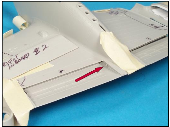
The metal strips were test fitted to be sure that nothing interfered with their positioning.
