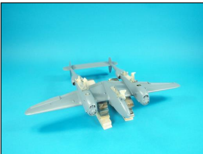
The entire aircraft was primed and a final check of the fuselage and wing surfaces was completed prior to applying the final paint colors.
