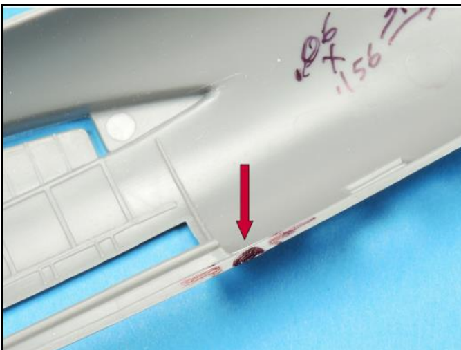
The gluing surfaces of the fuselage halves have raised areas which will need to be removed.
