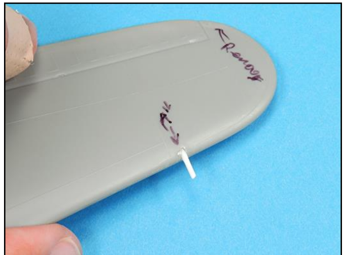
The pitot tube locations on the wings were filled in with .040 inch rod super glued into place, because the openings were too big. The openings were re-drilled with a .041 inch drill bit.
