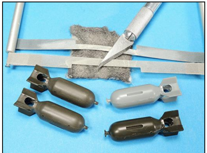
The bombs seam lines were carefully scraped, wet sanded smooth with a Flex-A File and then polished with a 0000 steel wool pad.
