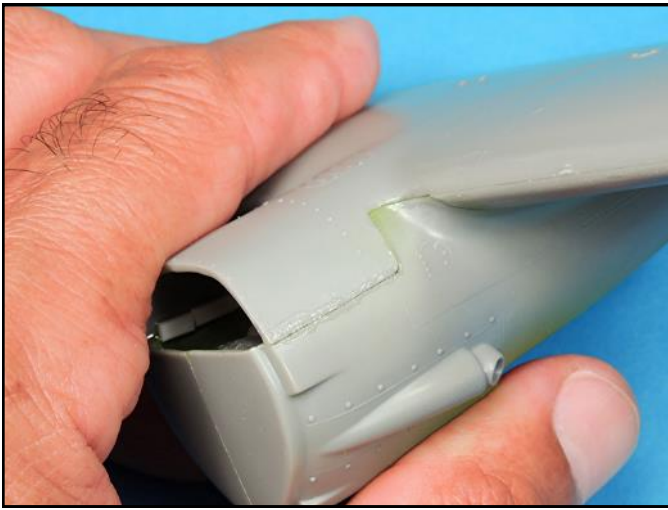
The super glue holds the gap closed, but scraping and sanding can weaken the seam.
