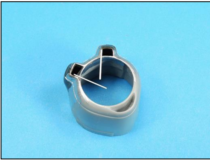
On this cowling assembly there were tiny voids in the front that were filled with .01 x .02 inch plastic strips.
