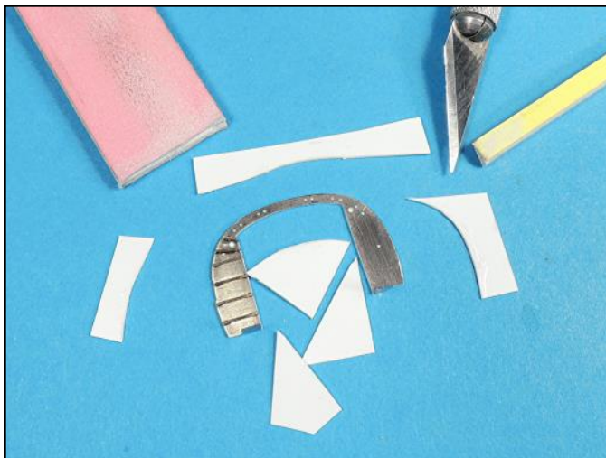
The Eduard forward cockpit bulkhead was laminated to a .015 inch thick plastic sheet to make it stronger.
