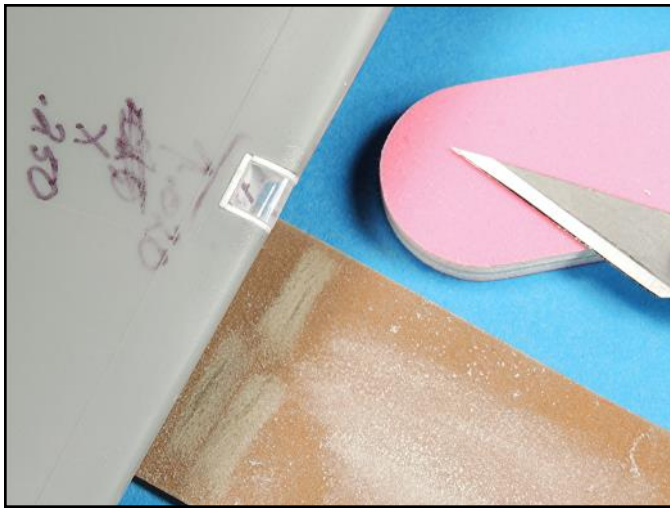
Careful sanding, shaping and form fitting of the wing light clear covers resulted in a tight fit on both wings.
