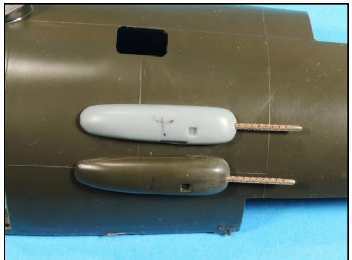
The positioning holes in the fuselage were enlarged to .065 inches to allow for some play so the gun packs could be properly positioned.
