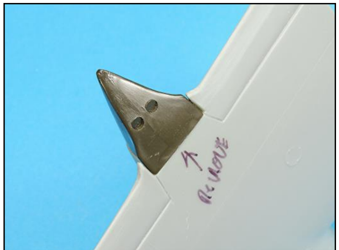
The trailing edge section of the engine nacelles have positioning tabs that need to be removed in order for these parts to sit correctly.
