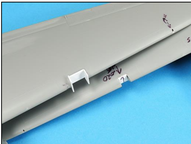
The wing light locations were boxed in with .02 x .188 inch strips super glued into place. Be sure that you apply a bead of super glue around the outer perimeter of each box.
