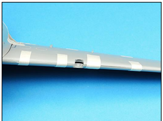
The leading edge lights on both wings have gaps, and the sides are misaligned.
