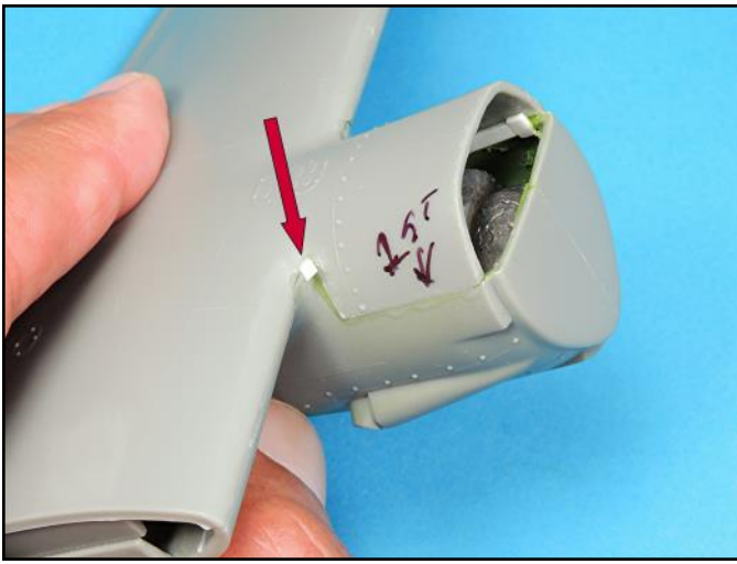
Small lengths of plastic of various thicknesses were slipped into the voids in the forward wing areas and then super glued into place.
