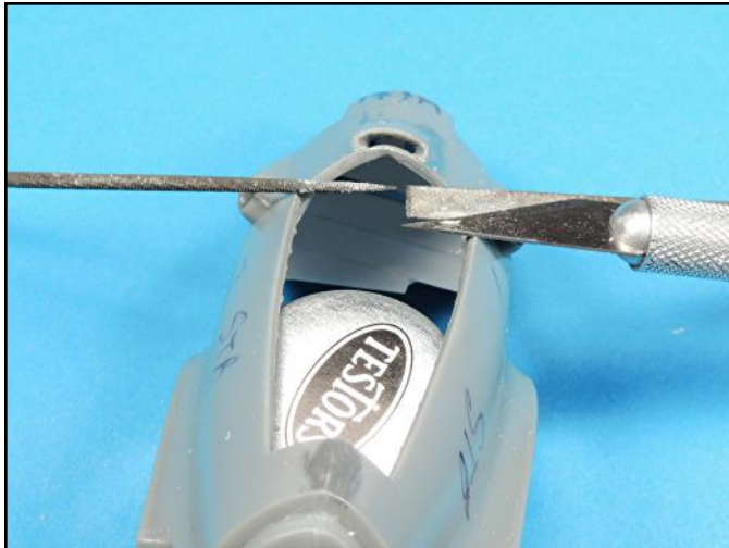
The openings were then carefully cleaned up and shaped with micro files.
