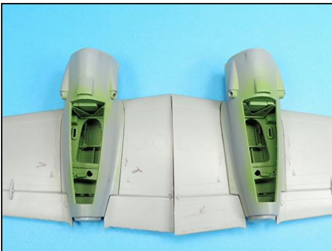
The nacelles have gaps on both sides that will need to be filled and sanded smooth.
