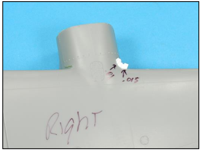
Beads of super glue were applied around the entire perimeters of these added strips using a .018 inch diameter wire as an applicator.
