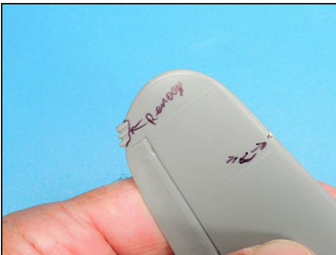
The trailing edge formation lights were badly misaligned between the upper and lower wings so they were sanded off.
