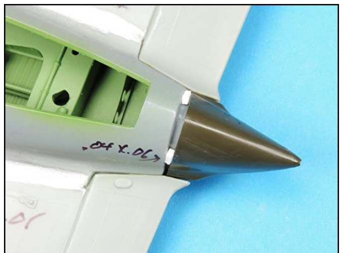
The proper positioning of these parts leaves a large gap on the lower surface. Small lengths of plastic were super glued into place to add strength to the assembly before filling the voids with plastic strips.
