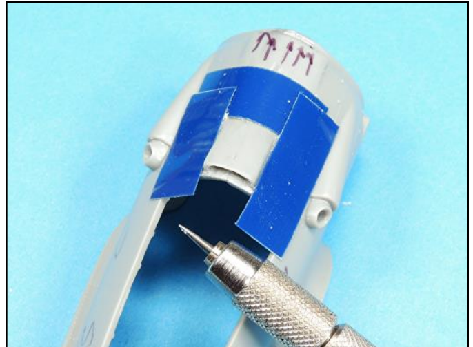
The edges of the air vents were then scribed to accent their attachments to the nacelles.
