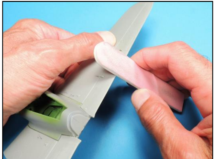
The trailing edge was scraped and wet sanded smooth with a sanding stick.
