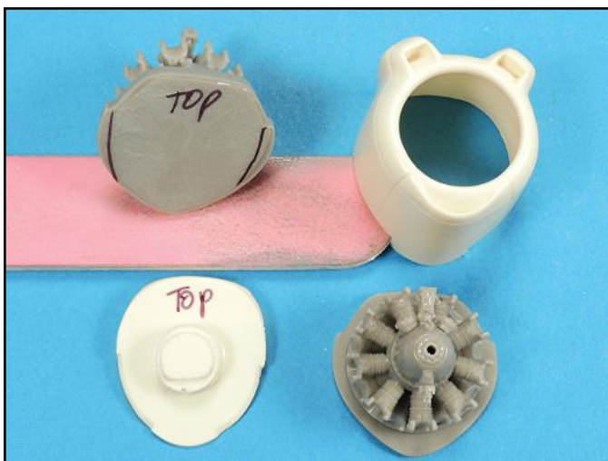
The Quickboost engines can be made to fit into the Loon Models cowlings by just tracing the outline of the Loon Models backing onto the Quickboost engine backing and then form fitting the engine into the cowl.
