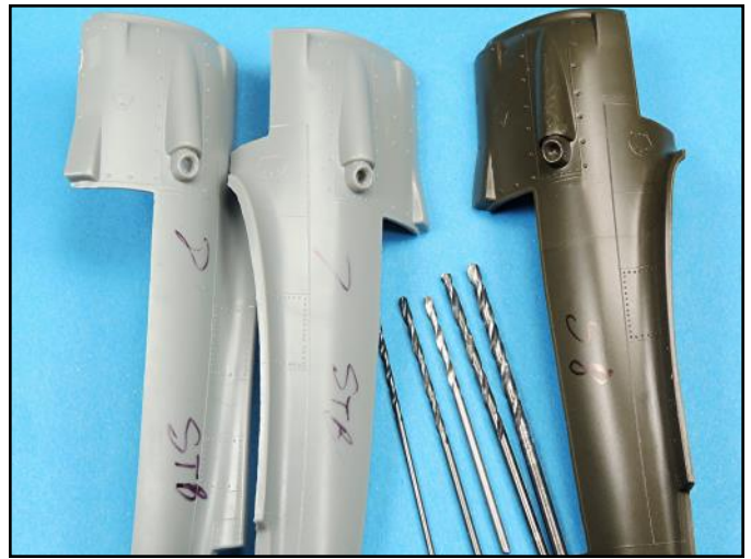
The engine exhausts were drilled deeper using progressively larger drill bit sizes. The four exhaust port openings were completed with a .086 inch bit (#44).
