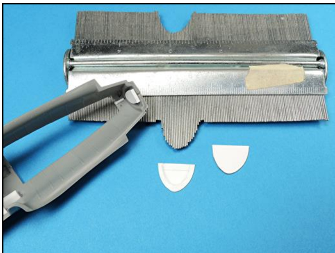
The aft interior area of each nacelle had noticeable framing that needed to be added. The framing shapes were made with a contour gauge, which was then traced onto .020 inch plastic and cut out.
