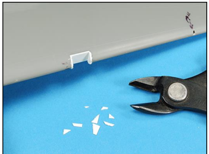
The excess plastic was trimmed with a pair of plastic cutters.
