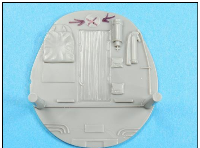
This large injection mark at the top of the cockpit bulkhead was removed with a length of sandpaper wrapped around a length of balsa wood.
