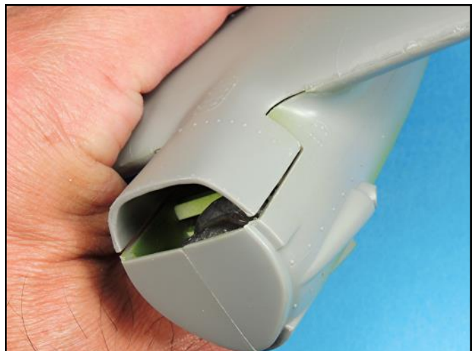
To fix the gaps between the upper and lower forward engine nacelles, they were pressed together and super glued.
