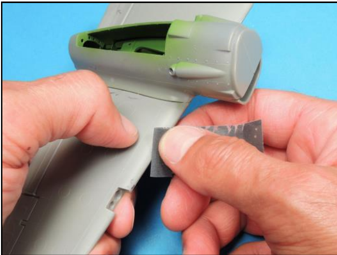
The leading edges of the wings were carefully scraped and wet sanded smooth.
