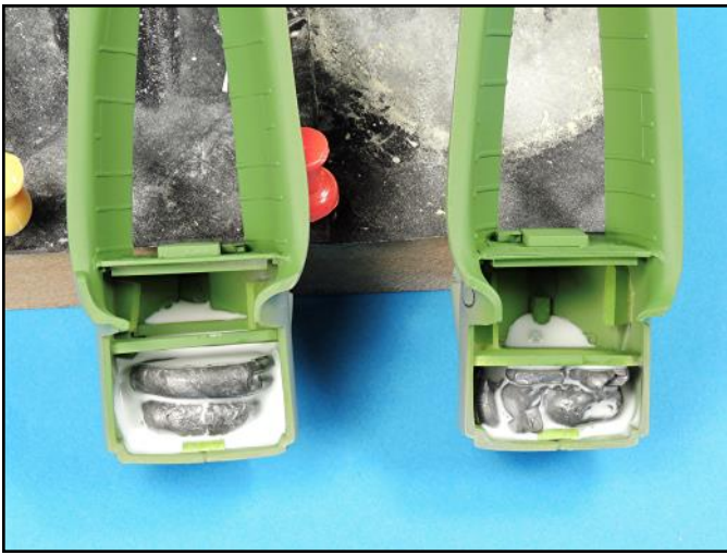
Mashed lead weight was inserted into the box areas of each nacelle and white glue added to secure the weights into place.
