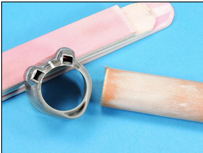
The engine cowling openings were reshaped using a 3/4 inch wood dowel with a 320 grit length of sandpaper wrapped around it.
