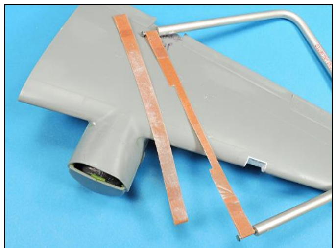
A Flex-A-File was used to smooth out the plastic around the contoured areas between the nacelles and the leading edges of the wings.
