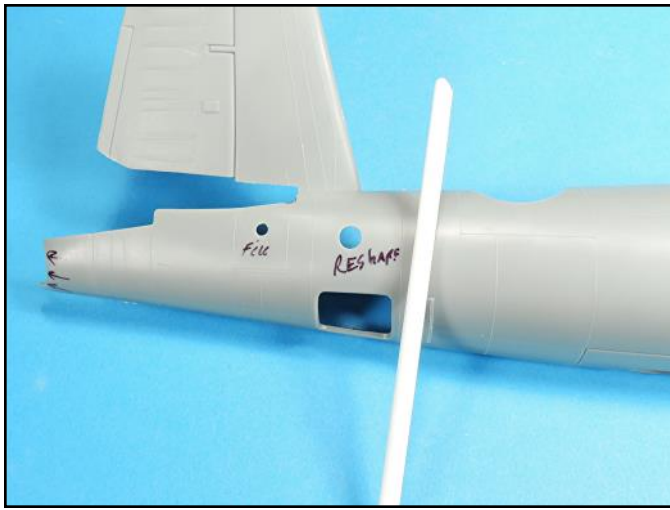
The clear parts for these openings are round, but the openings are not. Reshaping them was accomplished with a sanding rod.
