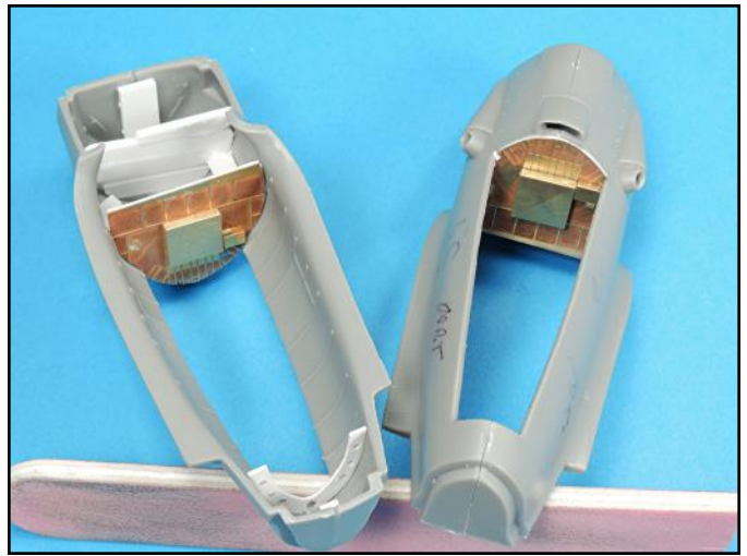
The engine nacelles are now ready for priming.
