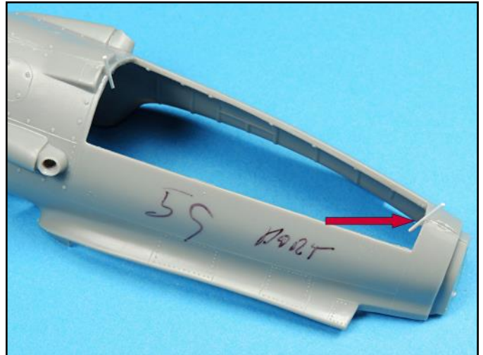
The edges of the nacelles were not square so after gluing the halves together, .01 x .02 inch strips were glued into place to fill these tiny gaps.
