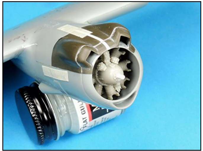
The engines were fit checked inside the cowlings and then taped to the nacelles to be sure there were no fit issues.
