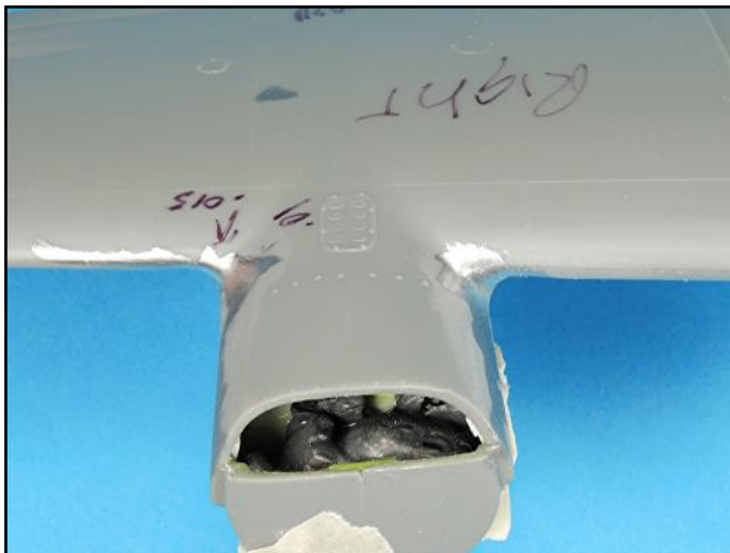
The contoured areas at the wing to nacelle connection points look good thanks to careful wet sanding with a Flex-A-File.
