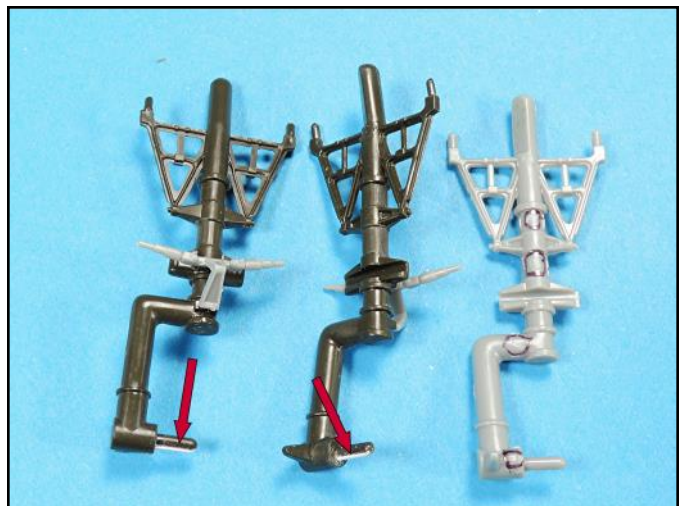
The fit of the main wheels to the landing gear was loose so tiny lengths of plastic (.01 x .02 inch) were glued to the axles to get a tight fit.
