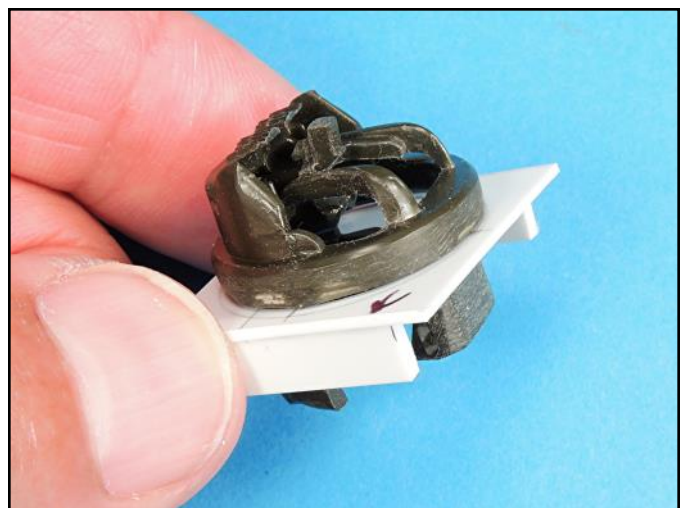
The hole should have some play in it so that the turret will just slide down into it. Note the reinforcing strips on the sides of the turret's positioned plate.
