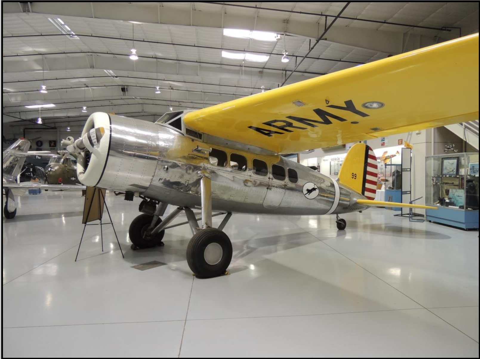
THIS LOCKHEED VEGA DL-1 ALL METAL AIRCRAFT IS LOCATED AT THE PIMA AIR MUSEUM IN TUCSON, ARIZONA. EARLIER VERSIONS OF THIS AIRCRAFT WERE MADE OF WOOD.
