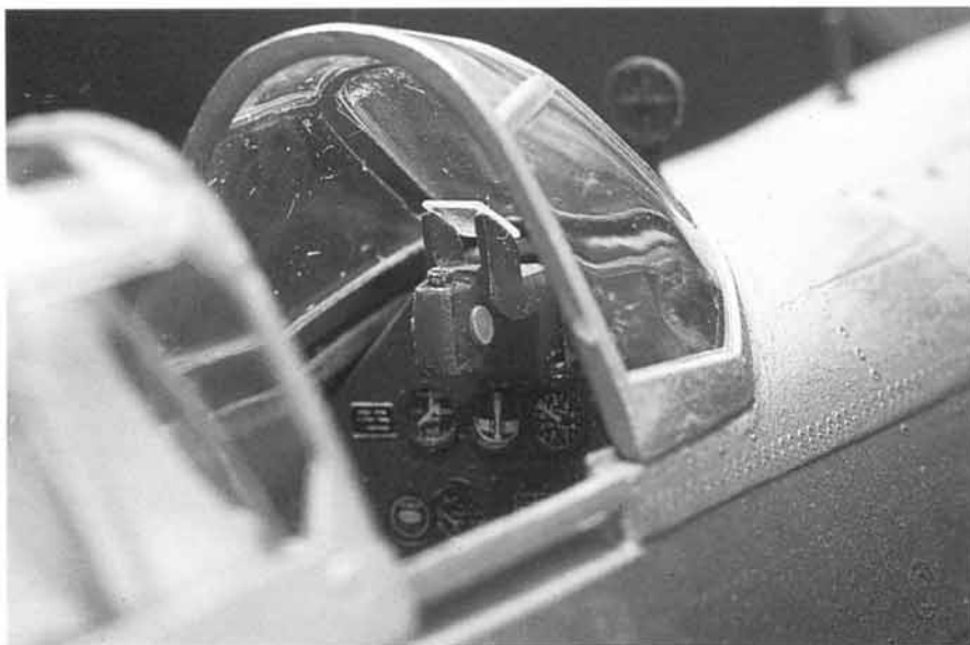
Revell's stock 1/32 scale P-40 gunsight, modified to sport reflective glass and adjusting dials. The disks were punched from sheet styrene with Waldron's punch tool.
