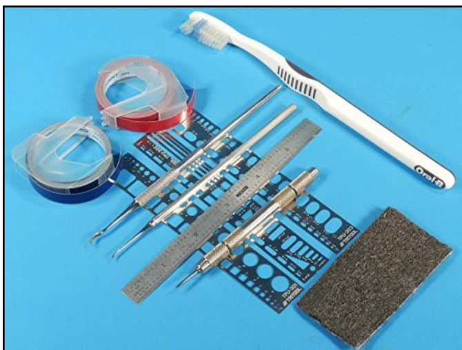
Here are the basic tools for restoring panel lines. Bare Metal Foil makes the best plastic scribe. The best templates for scribing are photoetch, which are very flexible. The needle scribe works great for restoring rivet detail.
