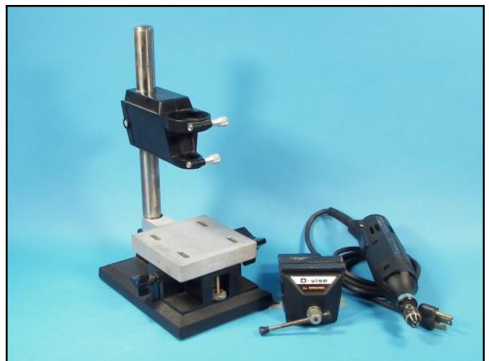
A variable speed motor tool, a Dremel drill press stand and a Dremel vise are the perfect combination for precise drilling. To hold plastic parts in the vise, sandwich the part between strips of balsa wood.
