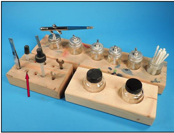
I like to keep my airbrushing tools in easy reach. Everything I need for an airbrushing session is stored in these three organizers. The arrow points to a .015 inch wire that I use to clear the airbrush head of paint while airbrushing.
