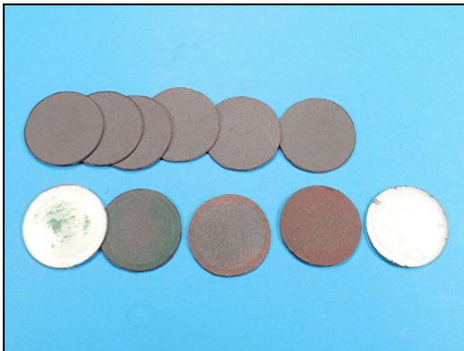
These cap seals are ready to replace worn white ones. Also, airbrush jars sometimes have thin styrofoam seals and these will dissolve when using enamels or lacquers, so remove and replace them with automotive gasket seals.
