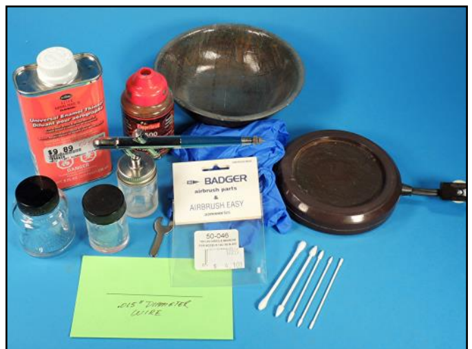
These are the essential tools for airbrushing. Always keep an ample supply of thinner and spare airbrush parts and jars. Copper BB's are great for mixing paint in its original jar. The shaped Q-Tips are made by Tamiya.
