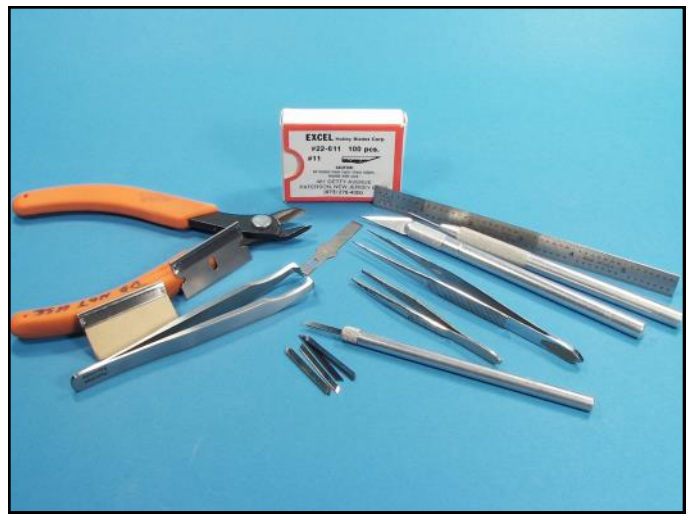
Here are the basic hand tools for snipping, cutting, trimming and scraping. The long black blades are stencil knives and the stainless steel sniper is a despruing tweezer cutter.
