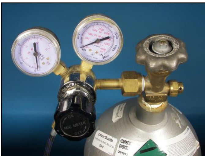
The regulator on my air supply tank has two gauges. The one on the right indicates the tanks air supply and the gauge on the left indicates the pressure of the air being supplied to the airbrush, which is controlled by the black knob.
