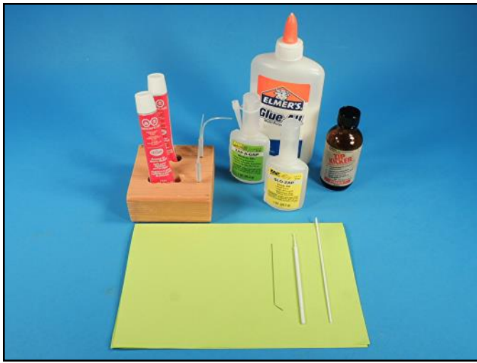
These are the three types of glues I like to use. I made the glue tube holder for the Testors red tube glue for upright positioning. The clear tubes to the right of the Testors glue are for precise super glue application.
