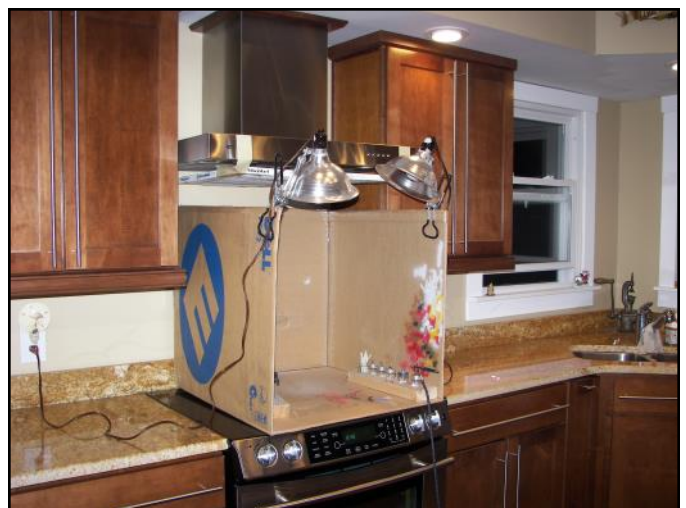
A spray booth can be as simple as a large box placed on top of a kitchen stove. This set up works great if the stove vent discharges to the air outside. To protect the vent from paint, tape an air conditioner filter to it.
