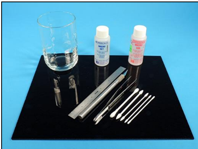
The black backed cutting board by "The Small Shop" was designed for cutting photoetch, but it also provides a nice contrast backing for cutting decals. Two part decal setting solution is a must for decal placement.
