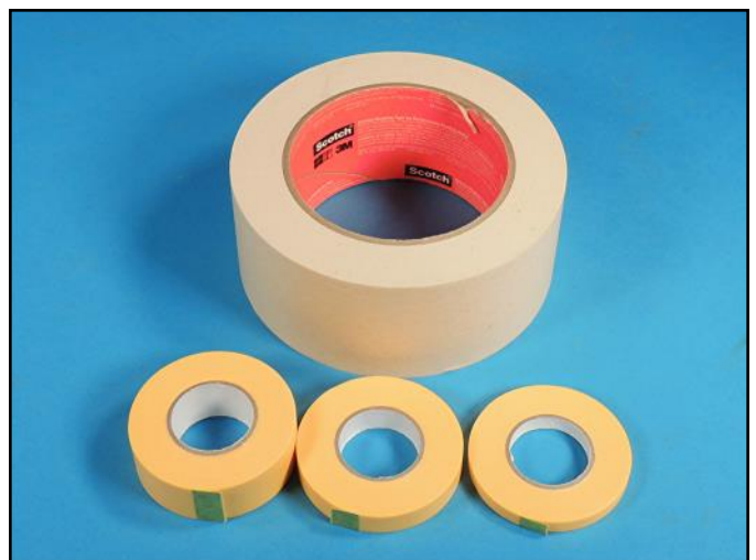
For taping parts together for fit checks, gluing and for masking, I like to use 3M painter masking tape #2050 and Tamiya masking tape.
