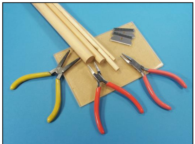
For cutting, bending and shaping photoetch, you will need dowels, flat faced needle nose pliers and single-edge razor blades. I found the red handled pliers in a jewelry supply store and they work great.
