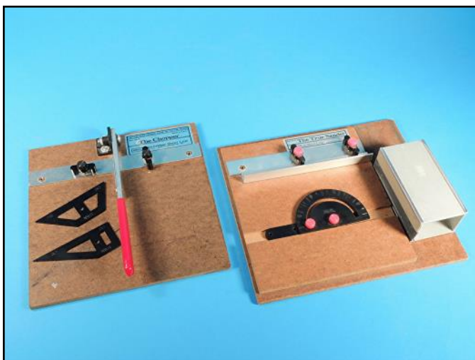
The Northwest Short line chopper and true sander are traditional model railroad scratchbuilding tools and they have a thousand uses in scale modeling. The chopper is especially handy when you need to make multiple parts.
