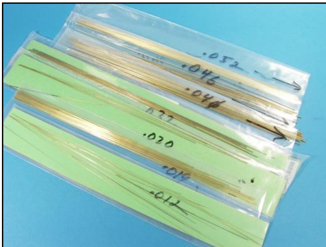
I keep a good supply of various diameters of stiff brass wire. It has a lot of uses such as cockpit and landing gear plumbing, engine wiring and landing gear brake lines.
