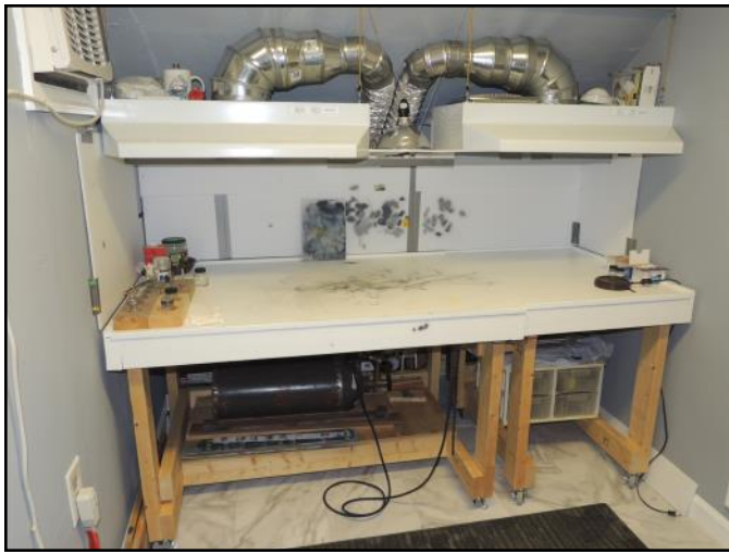
Here is my airbrush work station. It has dual 220-CFM vents and associated lightning. The foam board helps channel the air suction. I usually airbrush at a room temperature of 72 degrees or less and a humidity level of 55% or less.
