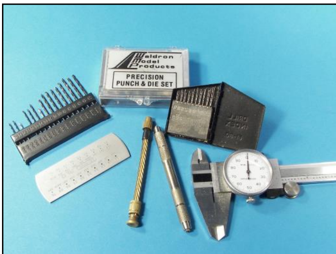
I keep a good supply of drill bits and I use a caliper to check diameters. A drill bit gauge is also a handy tool. The Waldron Punch has a thousand and one uses and twist drills make repetitive drilling easier.
